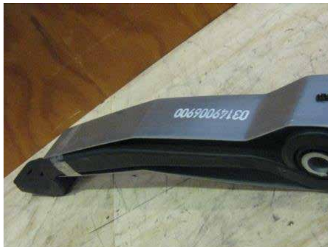
Example of a new arm complete with bush and safety retention device
