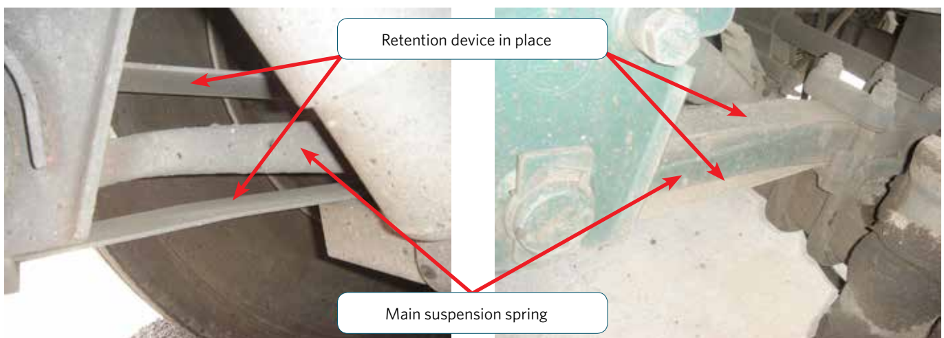
Example of a new arm complete with bush and safety retention device
