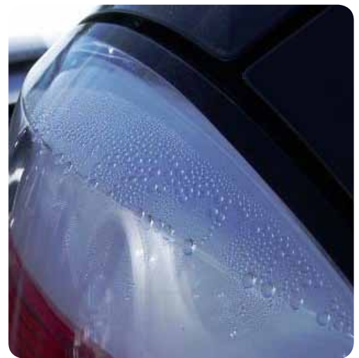
Figure 2: Heavy moisture - large droplets - FAIL
