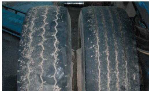
Incorrectly failed tyres: Both have highway rib pattern type
