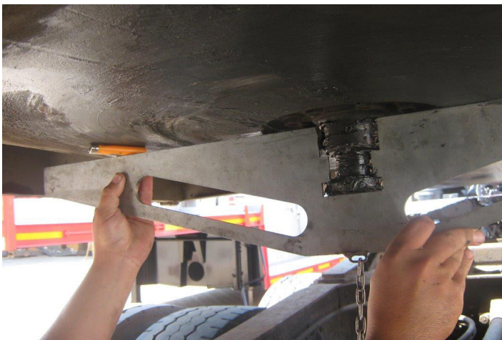
Checking for skid plate distortion
