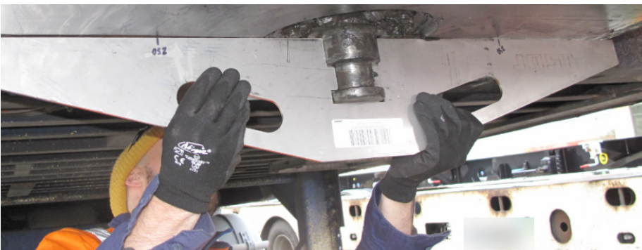
It's recommended to add measurements (such as the 250mm mark) to the gauge for quick reference.
