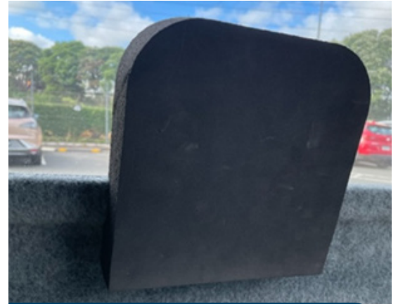
Suitable impact absorbing padding on a solid cargo barrier
