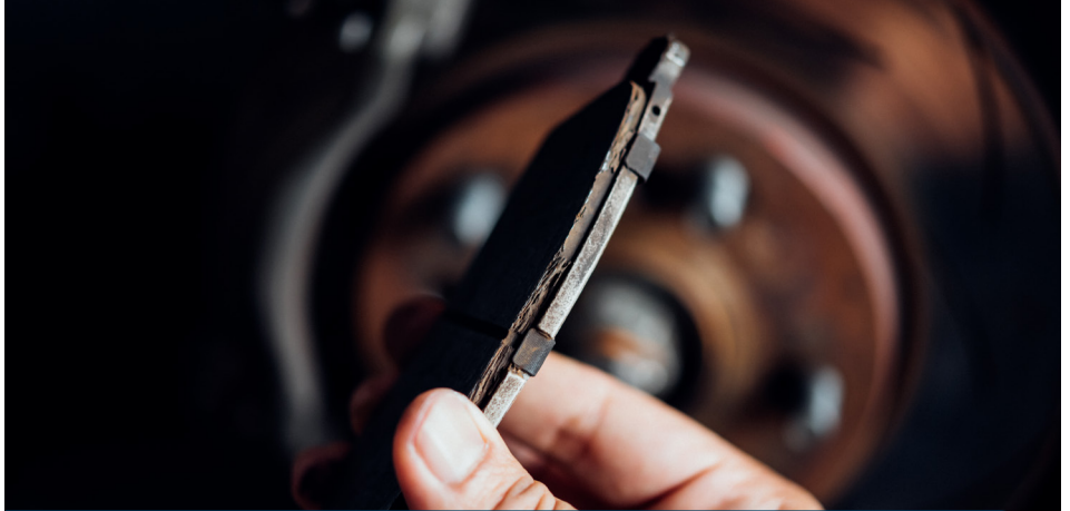
This is an example of a worn pad (removed from the vehicle for the photo) that is within manufacturers specifications and will most likely pass the brake test. However, this pad wouldn't last 12 months until the next inspection so a note or explanation to the owner should be made.
