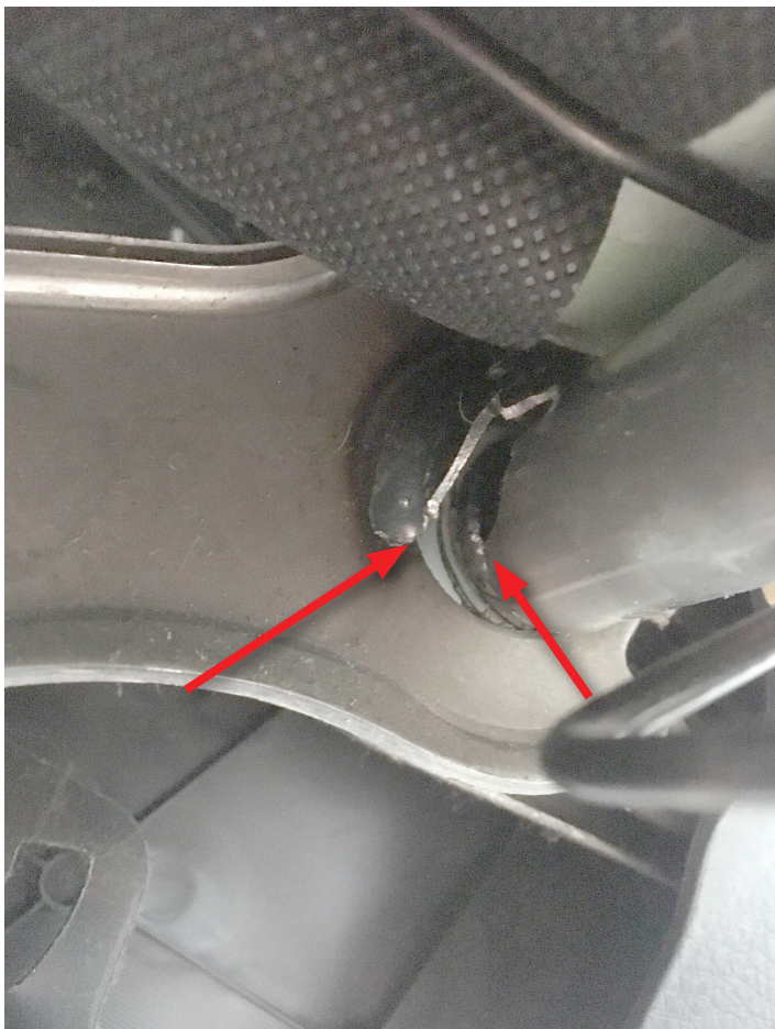
Example of base plate failure. Note that not all failures will be as large or obvious as the one in this image.
