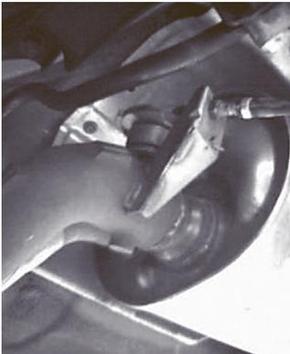
This setup doesn't meet the requirement that the exhaust system and silencer must be constructed so they cannot be readily interfered with. This vehicle must be failed for WoF.
