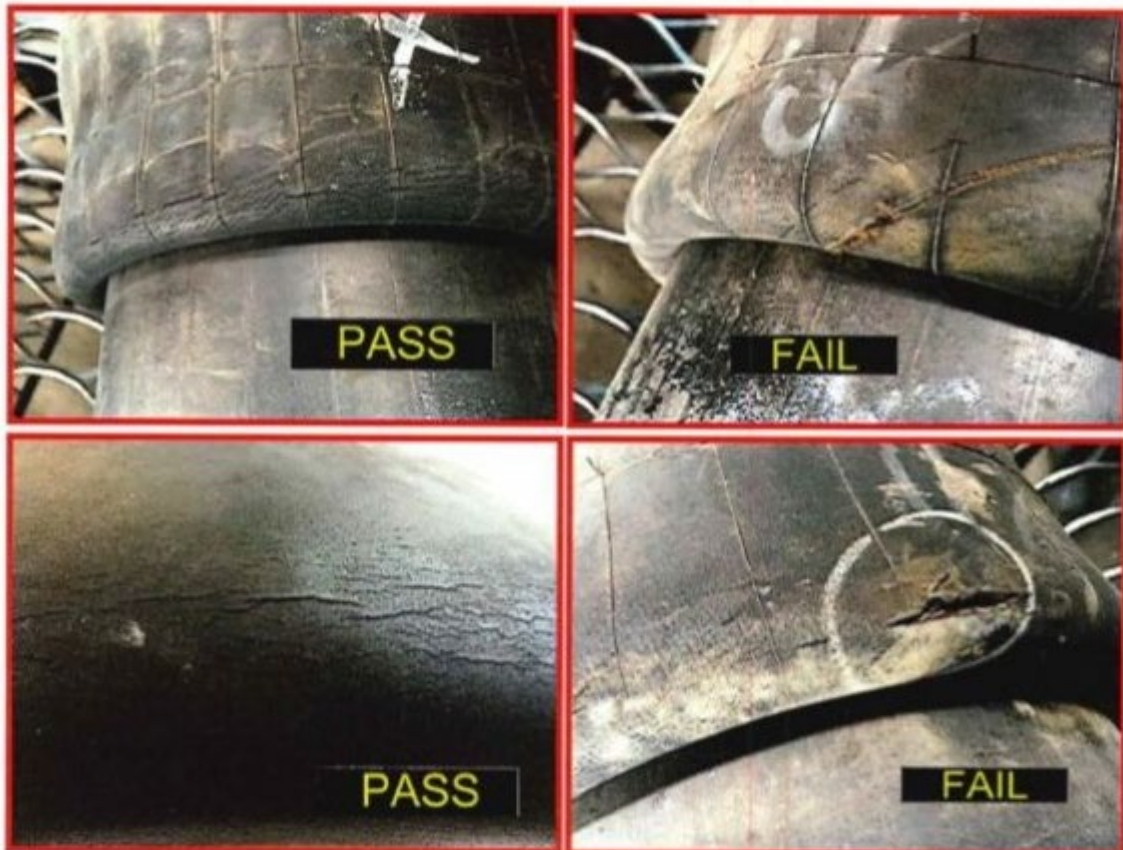
Figure 9-1-2. Sample air bag bellows images
