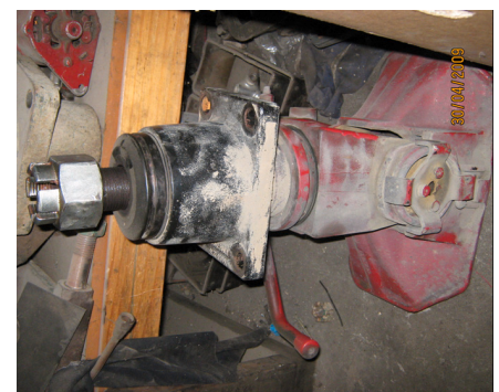
Picture showing the securing nut on a typical pin type coupling fitted to a drawbeam.
