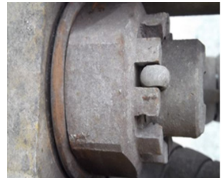
Picture showing signs of unserviceable tow-eye.
