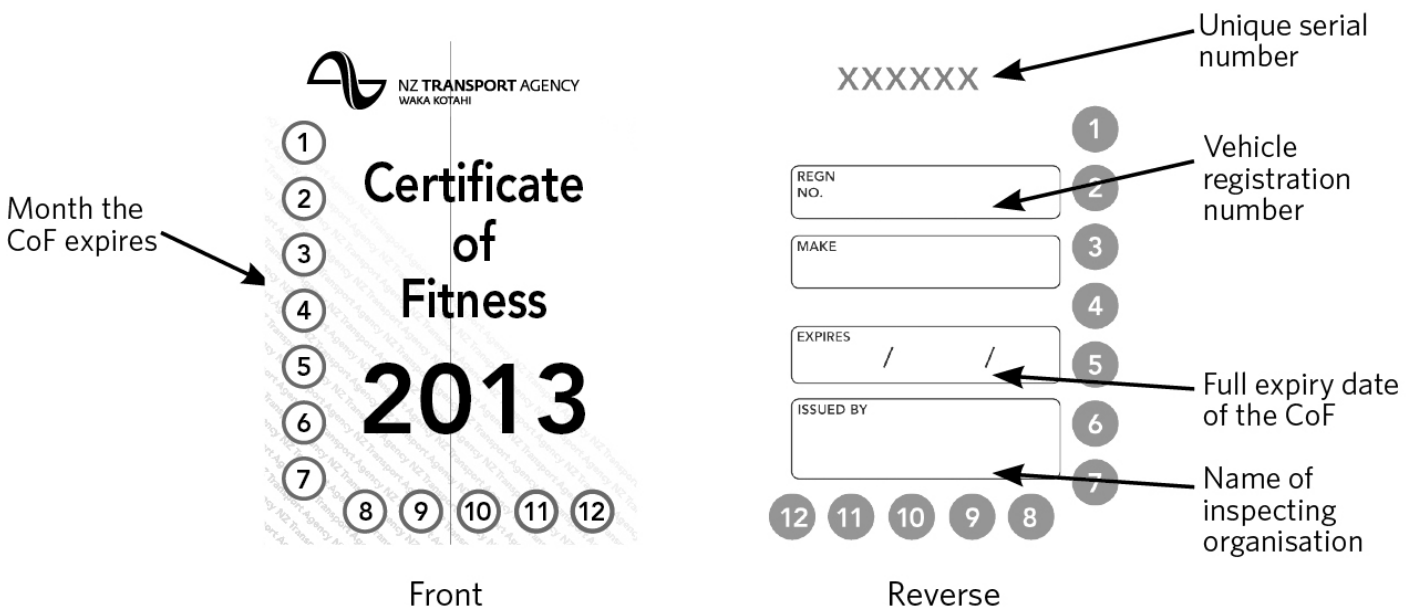
Figure 3-8-3. Certificate of Fitness (CoF) label details
